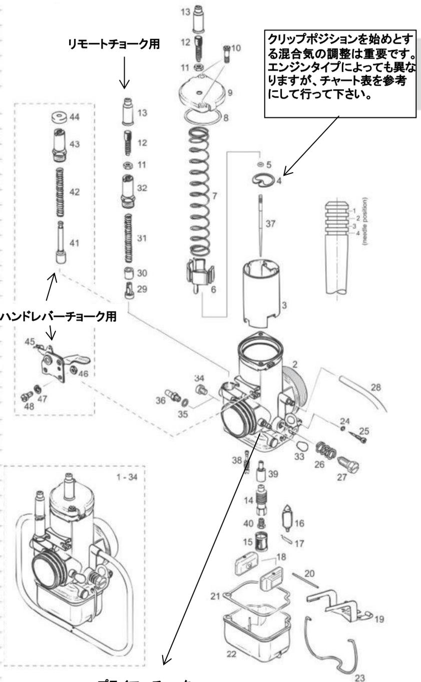
\*NOTE: a - Carburetor without calibration, c - Carburetor housing, not available as spare part, use carburetor assembly, d - Jet needle, see carburetor calibration sheet, e - Idle jet, see carburetor calibration sheet, f - Needle jet, see carburetor calibration sheet, g - Main jet, see carburetor calibration sheet, h - Only necessary on high altitude compensation kit.
